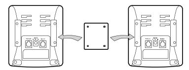
Connecting two expansion modules on a single host phone is shown as below:
