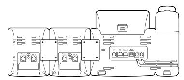
5. Connect the Ext jack on the host phone and the Ext in jack of the first module using one supplied cord. If you want to connect another module, connect the Ext out jack of the first module and the Ext in jack of the second module using one supplied cord. Connecting two expansion modules on a single host phone is shown as below:
